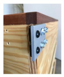
3. Grab four L-brackets. Attach a T-nut to the short side of each bracket (what would be the bottom of the L) with 2 1/2" 1/4x20 screws. Again, the raised side of T-nut should face away from bracket and the screws should go through the bracket first. Tighten the screws until they just begin to thread.
