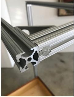
18. Use 1/2" <sup>1</sup>/<sub>4</sub>x20 screws to assemble one 6-holed flat bracket with 2 T-nuts, one in each hole at the bottom of the bracket. As usual, the screws should go through the flat bracket before the T-nuts, and the raised side of the T-nut should face away from the bracket.
