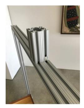
11. Assemble two more Lbrackets with T-nuts attached to each hole with 1/2" 1/4x20 screws. All Tnuts should be attached to the outside of the "L" with the screw heads on the inside.
