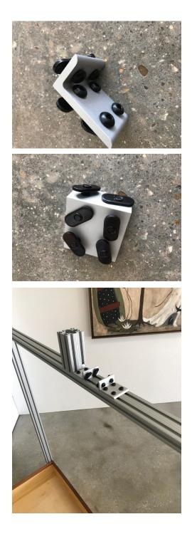
13. Slide the 15" metal beam between L-brackets with the exposed T-nuts while fitting into the beam's groove. The back of 15" beam should be flush with the edge of the 43" beam, and the round anchor hole on the beam should face the right side of the box.
