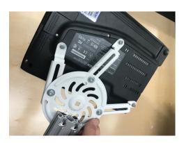
25. Using four zip ties, attach the Kinect sensor to the 11" metal beam so the sensor points downwards. The base of the sensor should point toward the back of the box. Tighten the ties so the sensor is snug against the beam. Make sure you do not cover up any of the sensors with the zip ties.
